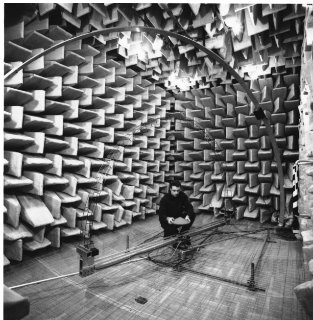
FIG. 1. Photograph of the automated goniometer for measuring hemispherical scattering being assembled in an anechoic chamber at the University of Salford. The lower part of the structure is covered with absorbent when operating.
